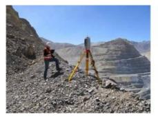
The RIEGL VZ-4000 laser scanner is capable of up to 222,000 measurements per second at a maximum range of 4,000 metres. In April 2012, the VZ-4000 toured the world to prove it, with demonstrations taking place in mines in both Chile and Russia.
