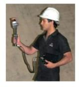
The ZEB1 mobile handheld laser mapping system has been proven to be able to outperform traditional terrestrial laser scanning during field tests in Chile. Supplied by 3D Laser Mapping and operated by Chilean company GEOCOM, the ZEB1 was used to conduct a survey of a stockpile in a covered mining facility.
