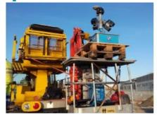
On behalf of the Emilia Romagna Railways (Ferrovie Emilia Romagna), Siteco is carrying out a verification project of the clearance outlines of the railways in this region of Italy. For the railway inspection, Siteco used the Road-Scanner 4 mobile mapping system associated with the Rail-SIT software application, expressly developed to optimize the analysis and inspection activities typical of
