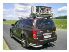
Gispro have successfully implemented Land Based Mobile Mapping System (MMS/MLS). The system consists of Riegl laser scanners, digital videoscanners and ground-penetrating radar. Positioning and orienation are established using POS420 and GPS receivers with IMU and DMI, built onto a car.
