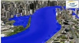
AAM's 3D Flood Simulation of Brisbane, Australia, was used extensively by Australian and Global media during the recent flood crisis in Brisbane. The flood level simulations were produced interactively in 3D. This was a very effective way of communicating the impact of the flood on buildings and infrastructure and it provided a valuable tool in assessing the potential risk for the city in the days leading up to and during the flood peak.
