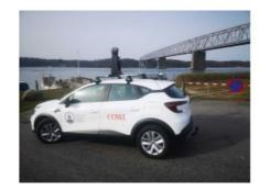
The Mosaic 51, a 360-degree mobile mapping camera, is now fully integrated with external GNSS to easily achieve real-time kinematic (RTK). Thanks to these extended capabilities, Mosaic's solution offers centimetre-level accuracy for customers with a high demand for precise position data.
