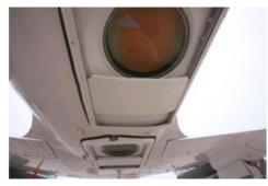
The Beechcraft King Air B200, owned by AELIS, is a multipurpose aircraft, capable of flying at a max speed of 280 knots and offering a max range of 1500 NM. It is modified under EASA approved STC and fitted with 2 holes of 52cm of diameter, ready to take on worldwide missions for photogrammetric and Lidar surveys.
