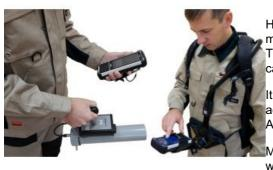
Handheld's Nautiz X8 ultra-rugged PDA has paired with the AT6101C backpack-style mobile spectrometer from Belarus-based ATOMTEX to aid in the detection of radiation. The AT6101C interacts with the Nautiz X8's GPS, GPRS, Wi-Fi and BT functionalities to capture and geo-reference data, then stores the data directly on the mobile unit.
