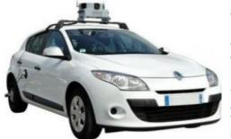
With the strong support of SBG Systems, ACTRIS tries to revolutionise GIS data collection method by releasing VIAPIX, a vehicle-borne image-base mapping system. The company chose the IG-500E for real-time image georeferencing. This miniature inertial sensor directly merges inertial data with GPS and odometer information to achieve the best performance. VIAPIX is a vehicle-borne mapping system.
