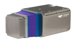
Teledyne Optech has announced that its newest compact Lidar sensor, Teledyne Optech's CL-360, is available for purchase through its second integration partnership with LiDARUSA. Optimized for UAV and mobile applications through industry-leading scan speed, vegetation penetration and small-object detection, the CL-360 has enabled LiDARUSA to design a product that offers premium performance, data quality and collection efficiency for UAV and mobile projects.
