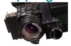
Leica Geosystems has announced the release of the <u>Leica SPL100</u> as part of the RealTerrain reality capture solution. It enables airborne professionals to more efficiently collect and process Lidar data of large areas, day or night and in leaf-on or leaf-off conditions.
