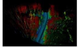
The invention of the Velodyne HDL-64 High Definition Lidar sensor, using 64 lasers contained within a fast-spinning unit to create a true threedimensional terrain map, is a new approach in the field of lidar technology.
