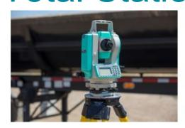
Nikon-Trimble has introduced a new version of the Nikon NPL-322+ total station, now available in both reflectorless and prism-only versions.
