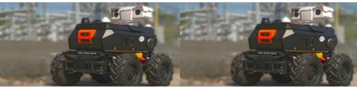
NV5 Geospatial has announced the debut of the ARIS II Rover, its upgraded robotic electric substation monitoring system. After five years of in-field implementation and testing, the rover meets the industry's most exacting standards for ruggedness and reliability. It is able to function in harsh environmental conditions and on the various terrains that are commonly found at distribution and transmission
