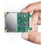
Topcon Europe Positioning, The Netherlands, has announced a light, ultra-compact dualfrequency positioning engine, the B110 GNSS receiver board for OEM applications. The B110 is the first GNSS board with Topcon's Vanguard ASIC, supporting 226 universal channels for GPS, GLONASS and Galileo tracking and scalable positioning from submetre DGPS to sub-centimetre RTK.
