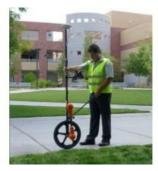
Optimal Ranging, Inc, (ORI, USA) has introduced the Spar, which is a handheld, onepass, remote sensor capable of locating and GIS mapping in 3D subsurface cable, conduit and pipe with up to centimeter-level accuracy to depths of one meter, decimeter-level accuracy to depths of three meters and sub-meter accuracy to depths of fifteen metres.
