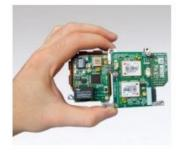
OxTS has announced the latest addition to the OEM line of inertial navigation systems aimed at system integrators. The xOEM500 is a GNSS/INS embedded on a single, compact board set and marks OxTS' smallest, lightest INS offering to date.
