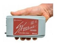
Geneq, Canada, has announced the SXBlue III-L GNSS, a palm-sized L1/L2/GLONASS GNSS receiver that is designed to use OmniSTAR's G2 or HP service to attain 10cm accuracy in all regions of the world.
