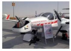
With the successful integration of SPECIM's AisaFENIX, a full spectrum imager, on the DA42 MPP special mission aeroplane, Diamond Aircraft Industries has added first-rate hyperspectral detection capabilities to its range of turnkey survey solutions. Diamond Aircraft Industries, Exogenesis and SPECIM teamed up to unite hyperspectral data capture and multipurpose data analysis options on the advanced DA42 MPP remote sensing platform.
