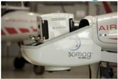
Diamond Aircraft, Austria, has introduced the new DA42 GEOSTAR that enables the collection of laser scanning and photo-grammetry data during one single flight. The team of Diamond Airborne Sensing (subsidiary of Diamond Aircraft) announced it has succeeded in perfect sensor integration on the DA42 MPP, the most economic remote sensing platform worldwide. Both systems are integrated with sufficient resources for fuel and flight crew.
