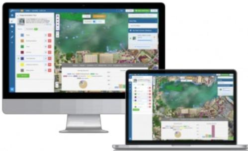
Picterra has introduced the custom detector, a tool that allows users of its online platform to build their own artificial intelligence (AI) models to detect objects in aerial and satellite images. The new tool allows users without any previous machine learning experience to create their own AI detection model and train it to identify their specific objects of interest in just a few steps.
