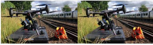
Plowman Craven has introduced Vogel Freedom, a UAV survey system designed for rail infrastructure surveying. Vogel Freedom is a survey-grade solution that surveys tracks without physical access. A novelty in the industry, the solution uses Plowman Craven's unique IP and offers benefits such as efficiency, safety and sustainability while maintaining Vogel's class-leading Band 1 survey accuracy.
