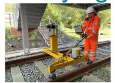
Plowman Craven has invested over GBP1 million in innovative technology to provide clients with a complete solution for rail surveying, from both the ground and the air. Plowman Craven is a leading surveying company in the UK.
