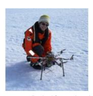
Engineers on board the Alfred Wegener Institute's research icebreaker *Polarstern* have programmed an unmanned autonomous vehicle (UAV), allowing it to navigate despite the deviations produced by the Earth's magnetic field near the North Pole. The researchers recently celebrated the multicopter's first successful autonomous flight and landing on an ice floe.
