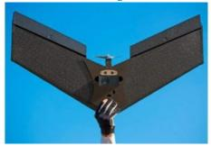
Lehmann Aviation (France) has launched the LA300, an automatic drone for professional, still aerial images (41MP) and video, for most accurate mapping and surveying. Designed for professional applications, including georeferenced orthomosaics and digital elevation models (DEM), the LA300 achieves professional imaging using the Nokia 1020 smartphone camera.
