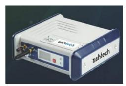
Ashtech, France, has released version 3.5 firmware for the ProFlex 500 GNSS receiver that includes a powerful NTRIP Caster to enable surveyors, municipalities, mining, engineering and agricultural operations to easily implement and control their own very cost-effective and secure corrections network via NTRIP protocol. Ashtech dealers are also expected to take advantage of the new Caster feature to set up their own service network for their customers.
