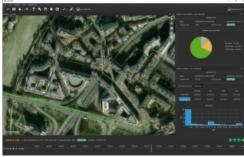
SBG Systems' popular INS/GNSS PPK software called Qinertia now covers all surveyors' projects by offering a licence dedicated to GNSS post-processing, according to the France-based company. Open to the world, Qinertia supports all major GNSS receivers and is now open to third-party IMUs.
