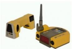
Topcon's RC-4 is a new, compact QuickLock remote system that integrates an array of advanced technologies that increases productivity on survey projects. The RC-4 uses dual lasers, a built-in spread-spectrum radio and Topcon's QuickLock technology to create on-the-job efficiencies from stakeout to topo and from construction layout to as-built surveys.
