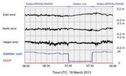
Since the launch of the last two Galileo satellites in autumn 2012, Fugro has been looking forward to demonstrating real-time Precise Point Positioning (PPP) based solely on Galileo signals. These two satellites have brought the constellation to a total of four satellites, the minimum required to permit calculation of a Galileo-only position. Fugro achieved this task on 18 March 2013, which was within one week of all four Galileo satellites being activated.
