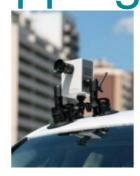
Imajbox, an integrated, portable and stand-alone surveying and mapping solution, has been completely renewed. The solution aims to stretch the limits of mobile mapping technology by making data capture accessible to any organisation. imajbox L, imajbox S and imajbox T can be used for roadways, railways, urban areas or trail surveys.
