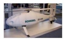
RIEGL Laser Measurement Systems and Applanix Corporation have announced that the Applanix AP50 GNSS-Inertial sensor system was successfully integrated with RIEGL's VQ-820-GU topo-bathymetric airborne laser scanner on board the Schiebel CAMCOPTER S-100 UAV. The RIEGL VQ-820-GU is specifically designed to survey sea beds or the grounds of rivers or lakes, and is well suited for combined land and hydrographic airborne survey.
