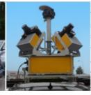
Siteco Informatica has delivered a Road-Scanner4 mobile mapping system to Amberg Technologies in Switzerland. This RoadScanner features the flexibility of using Lidar sensors from different manufacturers with fast in-field sensor changeover capability and a spherical camera system to be used for a wide variety of high-precision road and rail applications.
