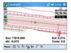
SBG (Sweden) has released Stringline model software which produces a complete 3D model representing any type of road. It is an all new reference type that uses parallel stringlines.
