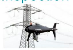
Schiebel, FLIR and Transpower have announced the successful demonstration of the Schiebel CAMCOPTER S-100 Unmanned Aerial System with the integrated FLIR Corona 350 sensor being used to inspect high-voltage power lines and supporting structures. This event marked the first time that this new capability was demonstrated using a UAS.
