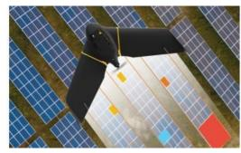
senseFly, a leading provider of fixed-wing drone solutions, has introduced the <u>senseFly Solar 360</u>, the latest addition to its senseFly 360 solutions range. Created in collaboration with software company <u>Raptor Maps</u>, this offering is a uniquely efficient thermal drone solution that enables the automatic assessment of solar plant performance at a submodule level.
