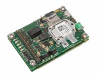
Septentrio, a leading global supplier of high-accuracy positioning technology for demanding applications has announced today a new addition to their GNSS/INS portfolio. AsteRx-i S UAS combines GNSS technology with industrial-grade inertial sensor to provide high-accuracy, reliable positioning and 3D orientation (heading, roll, pitch) to aerial drones and other compact robotic systems.
