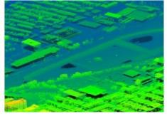
In response to the growing use of Lidar, photogrammetry software developer SimActive has integrated a new Lidar workflow in its Correlator3D product. The capability enables users to import a point cloud in the software and to perform registration with an image dataset. Using Lidar as control eliminates the need for traditional ground control points (GCPs) during image processing.
