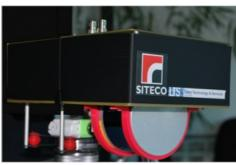
Siteco Informatica has launched its new high-performance Sky-Scanner Lidar and image data collection system for unmanned aerial vehicles (UAVs). In development since early 2015, the Sky-Scanner has already exceeded all performance expectations on the <u>DJI-S1000</u> and <u>DJI Matrice-600</u> airborne platforms.
