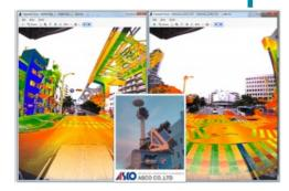
Over 120 kilometres of roadway infrastructure on the Japanese island of Okinawa were captured in February 2015 in high-accuracy 3D detail using SITECO's RoadScanner4 mobile mapping system equipped with Zoller & Frölich Profiler 9012 scanners and an iXBlue Landins inertial navigation system. The system is complemented with spherical colour imagery from Point Grey's LadyBug5 camera.
