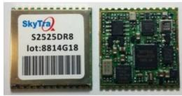
SkyTraq, a Taiwan-based GNSS positioning technology company, has introduced the all-in-one S2525DR8 GNSS dead-reckoning module with onboard integration of MEMS sensor and interface logic. The module is especially suitable for road vehicles requiring high accuracy and 100% positioning availability.
