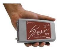
Geneq has introduced its smallest GPS L1/L2 OmniSTAR receiver. The SXBlue III-L is designed to use OmniSTAR's HP service to attain decimetre accuracy in all regions of the world including North/South America, Australia, Asia, Africa, Europe, and the Middle East reinforcing Geneq's "Go Real-time, All the Time†strategy.
