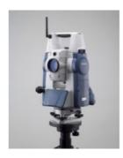
Sokkia (Japan) has released the Automated 3D Station NET05 offering high accuracy for industrial, construction and deformation monitoring applications. The NET05 provides 0.5" (0.15mgon) angle measurement accuracy using a combination of IACS (Independent Angle Calibration System) technology and absolute encoders enhanced with market proven RAB code (RAndom Bidirectional code) technology.
