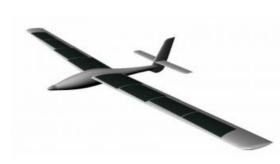
At the Esri International User Conference Imaging and Mapping Forum, Flightline Geographics has announced the first solar-powered UAS specifically designed for professional mapping applications. By integrating solar panels within the wings, flight times have doubled allowing much larger areas to be mapped in a single flight.
