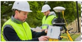
Spectra Precision has introduced its SP90m multi-frequency and multi-application GNSS receiver. The SP90m is a powerful, highly versatile, ultra-rugged and reliable Global Navigation Satellite System (GNSS) positioning solution for a wide variety of real-time and post-processing applications. It features integrated communications options such as Bluetooth, WiFi, UHF radio, cellular modem as well as two MSS L-band channels to receive Trimble RTX correction services.
