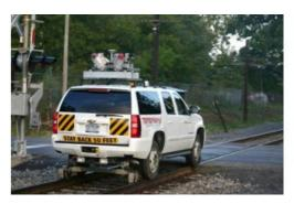
Mobile mapping system StreetMapper has been used to collect design-grade 3D data for a rail improvement project in New York, USA. Supplied by 3D Laser Mapping, StreetMapper uses a series of vehicle-mounted laser scanners to collect data at speed and with minimal risk to survey personnel. Selected by engineering firm CHA and operated by service provider Terrametrix, the StreetMapper system was chosen as a rapid and more cost-effective alternative to a conventional track survey.
