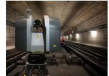
GeoNext has used Trimble technology to survey the Schiphol Tunnel and provide measurements as the basis for a 3D model to support essential railway maintenance and upgrades. Millions of passengers pass through the Schiphol Tunnel every year; it is a vital transport link between central Amsterdam and Schiphol Airport in the Netherlands. The speed and precision of the laser scanners
