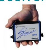
Geneq has launched an ultra-small SXBlue GPS L1/L2 dual-frequency GPS RTK receiver for high accuracy positioning. One of the smallest dual-frequency RTK GPS receivers in the world, weighing only 268g (~1/2 lb) and having dimensions of 11.26cm x 8.54cm x 3.53cm (4.43" x 3.36" x 1.39"), the SXBlue L1/L2 GPS is designed to be mounted on vehicles and use the vehicle power for machine control applications such as agriculture, mining, construction and other high-precision applications.
