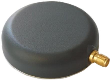
Tallysman has introduced the TW2920 antenna for simultaneous reception of L-band correction signals and all of the upper band GNSS signals including GPS L1, GLONASS G1, Galileo E1, and BeiDou B1. The TW2920 1dB bandwidth covers 1525MHz to 1559MHz for the L band down-link and 1559MHz to 1610MHz for the upper band GNSS.
