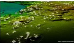
Teledyne Optech's Titan sensor was used by the University of Houston's National Center for Airborne Laser Mapping (NCALM), USA, to reveal extensive Mayan ruins in Guatemala. Lidar technology was able to identify hundreds of previously unknown structures, including raised highways and complex irrigation and terracing systems.
