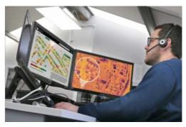
Using a high-tech thermal imaging camera to measure heat loss from roofs, aerial mapping company Bluesky International is helping to identify poorly insulated homes and other public buildings.
